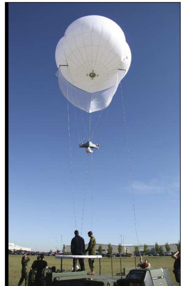
A tethered balloon with a suspended camera floats over the Edmonton garrison as part of ongoing Army training in observing, deterring and defeating insurgents who plant IEDs in Afghanistan.
